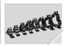
AERON Trefoil Clamps / Cable Cleats are used for laying single core cables in Trefoil touching formation which helps to maintain magnetic symmetry thereby avoiding electromagnetic heating and loss of current.
