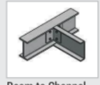
Beam to Channel
