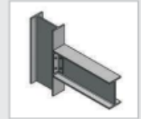
Beam to Beam
