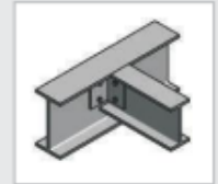
Beam to Beam
