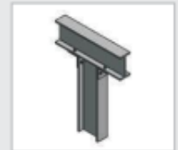
Beam Over Beam
